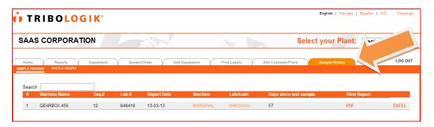
1. Clicking on the first sub-menu, also called **SAMPLE HISTORY**, allows disclosing all the results of all the oil tests made on a piece of equipment in Excel format.
